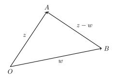
In the diagram, due to the triangular inequality, we must have  $AB \leq OA + OB$ , and hence  $|z - w| \leq |z| + |w|$  as desired.
